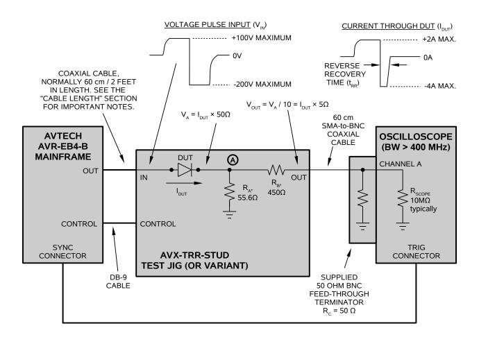
A 50 Ohm resistance (R<sub>C</sub> in the diagram above) must be connected to ground on the output. This can be a discrete resistor, a feed-through terminator, or the input impedance of an oscilloscope. If a high-speed sampling oscilloscope is used, the input should be protected by adding attenuator on the input. In the diagram above, the 50 Ohm feed-through terminator supplied with the AVR-EB4-B is used to provide the required 50 Ohm resistance.
