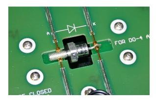
To install the diode, spread apart one pair of spring pins with your fingers or tweezers, and insert one end of the diode. Repeat on the other end.
