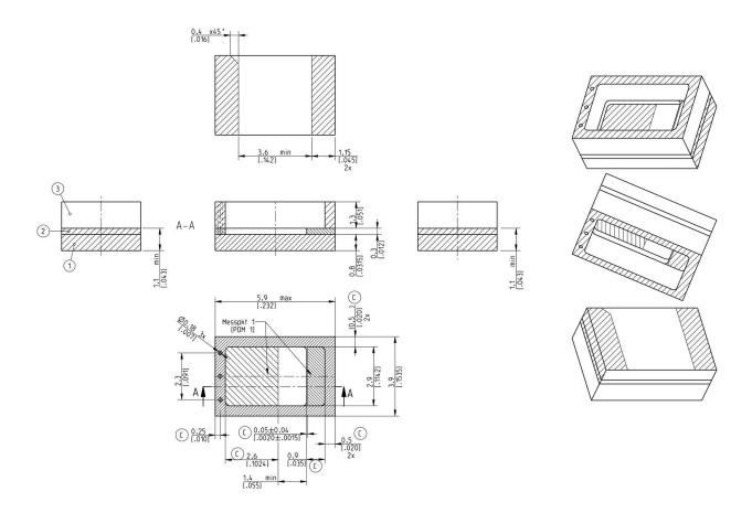
Probe points on the jig contact the two  $1.15 \times 3.9$  mm pads on the flat bottom surface of the package. One of these pads must connect internally to the device anode, and one to the device cathode.
