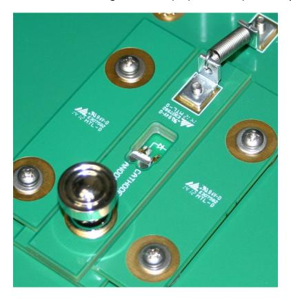
The anode pad must contact the left probe point, and the cathode pin must contact the right probe point.
