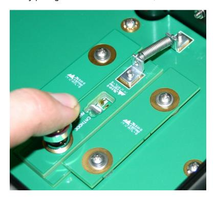
The DUT is then placed in the area immediately in front of the two fixed probe points, as shown in the photo above. Then slowly release the chrome knob, allowing the
