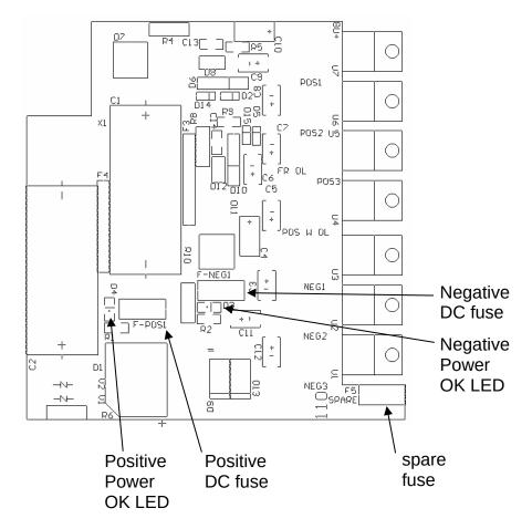
The positive fuse and one of the spare fuses on this circuit board are 1A slow-blow fuses, Littlefuse part number R452001. (This fuse can be ordered from Digikey, www.digikey.com. The Digikey part number is F1343CT-ND). The negative fuse is a 0.5A slow-blow fuse (Littlefuse R452.500, Digikey part number F1341CT-ND).
