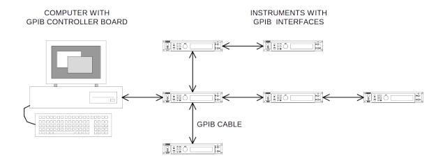
More than one computer controller can be present on the bus, if desired. Each device on the bus has its own address, in the range of 0 to 30.
