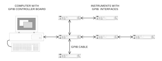
More than one computer controller can be present on the bus, if desired. Each device on the bus has its own address, in the range of 0 to 30.
