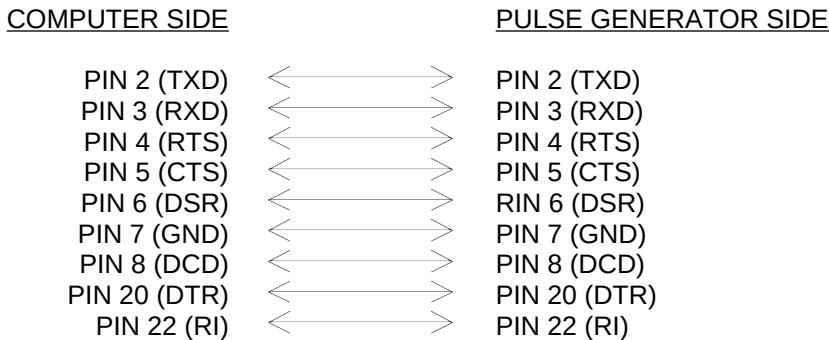
For computers with a 9-pin RS-232 connector, a "straight-through" cable is wired as shown below:
