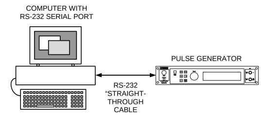
The computer is connected with a RS-232 "straight-through" cable. This cable is available at most computer stores, and it is the same type of cable that is generally used to connect a PC to an external modem. Beware that newer PCs generally have 9-pin male RS-232 connectors, whereas older computers generally have 25-pin male RS-232 connectors. The actual cable wiring connections are described in the "Cable Connections" section.
