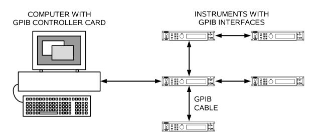
More than one computer controller can be present on the bus, if desired. Each device on the bus has its own address, in the range of 0 to 30.
