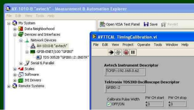
The Avtech pulser, in contrast, is connected with standard ethernet cabling, and is addressed in the LabView VI as "TCPIP::192.168.0.62". The pulser is also automatically detected in the Measurement and Automation Explorer tool, where it has been auto-assigned the alias "avtech" (which could have been used in the LabView VI, instead of "TCPIP::192.168.0.62").
