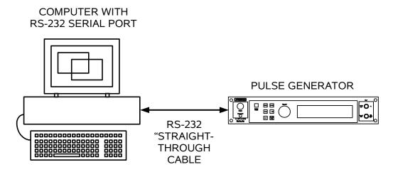
The computer is connected with a RS-232 "straight-through" cable. This cable is available at most computer stores, and it is the same type of cable that is generally used to connect a PC to an external modem. Beware that newer PCs generally have 9-pin male RS-232 connectors, whereas older computers generally have 25-pin male RS-232 connectors. The actual cable wiring connections are described in the "Cable Connections" section.
