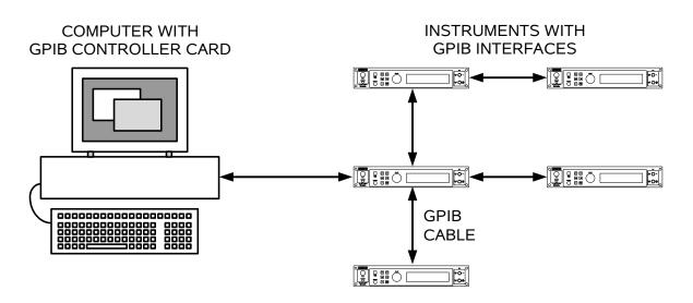
More than one computer controller can be present on the bus, if desired. Each device on the bus has its own address, in the range of 0 to 30.
