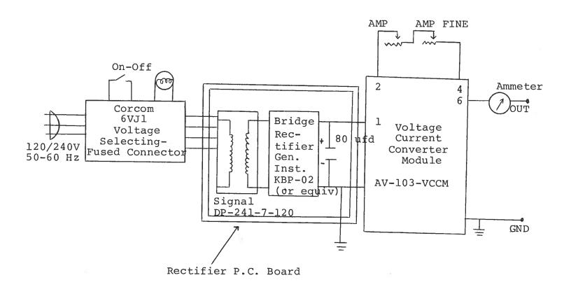
In the event that the AV-103 unit does not provide an output or is not operating properly as a constant current source, the cause and defective component may be identified as follows:
