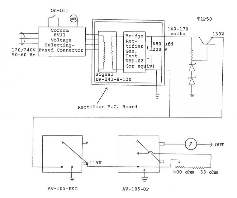
In the event that the AV-105 unit does not provide an output or is not operating properly as a constant current source, the cause and defective components may be identified as follows:
