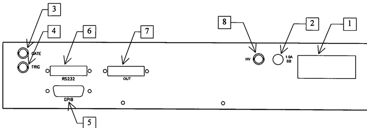
1. **AC POWER INPUT.** A three-pronged recessed male connector is provided on the back panel for AC power connection to the instrument. Also contained in this assembly is a 2A slow blow fuse and a removable card that can be removed and repositioned to switch between 120V AC in and 240V AC in.
