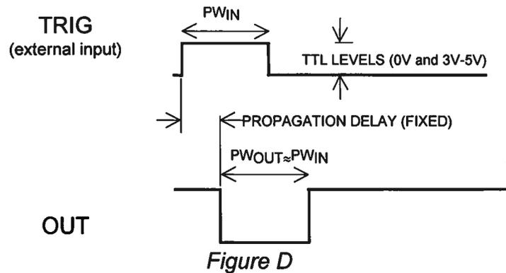
The delay, pulse width, and frequency (when in the internal mode), of the OUT pulse can be varied with front panel controls or via the GPIB or RS-232 computer interfaces.
