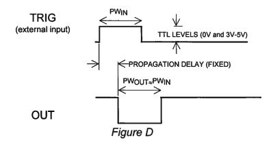
The delay, pulse width, and frequency (when in the internal mode), of the OUT pulse can be varied with front panel controls or via the GPIB or RS-232 computer interfaces.
