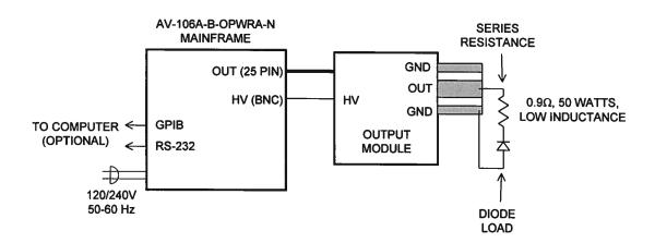
The loads can be connected (soldered) to the microstrip transmission line that protrudes from the output module.
