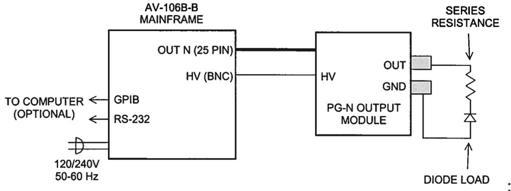
Both of these figures show a resistance in series with the laser diode. Since the AV-106B-B is a current pulser, this resistance is optional - it is not required for current limiting.
