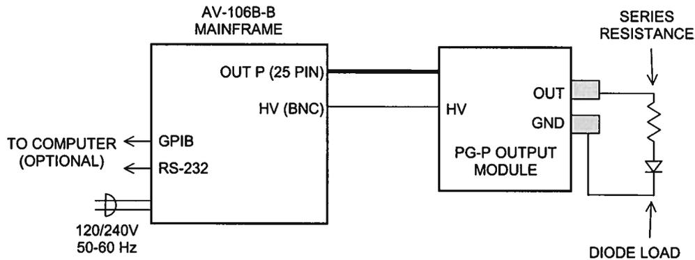
A typical connection scheme is shown below for negative output modules, supplied with “-N” and “-PN” units:
