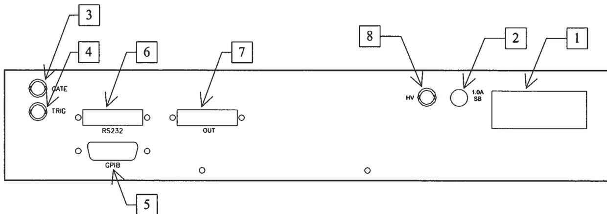
1. **AC POWER INPUT.** A three-pronged recessed male connector is provided on the back panel for AC power connection to the instrument. Also contained in this assembly is a 1A slow blow fuse and a removable card that can be removed and repositioned to switch between 120V AC in and 240V AC in.
