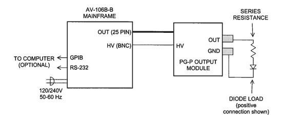
The loads can be connected across the banana posts on the output module.
