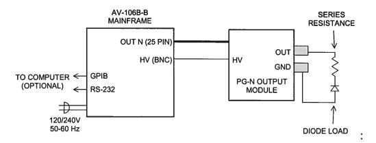
Both of these figures show a resistance in series with the laser diode. Since the AV-106B-B is a current pulser, this resistance is optional - it is not required for current limiting.
