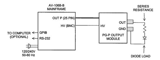
A typical connection scheme is shown below for negative output modules, supplied with "-N" and "-PN" units:
