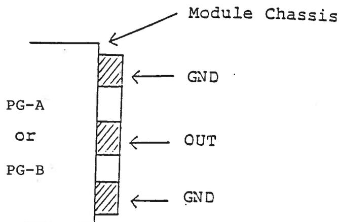
The load should be connected between the OUT and GND terminals using very short leads ( $\ll$  0.5 cm). (See 11).
