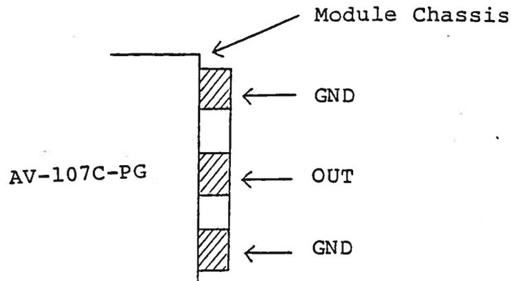
The load should be connected between the OUT and GND terminals using very short leads ( $\ll 0.5$  cm). The voltage across the load may be monitored by connecting a length of 80 mil semi-rigid 50 ohm cable as shown below (or by means of a high impedance scope probe). The current may be monitored using a current probe such as the TEKTRONIX Model CT-2.
