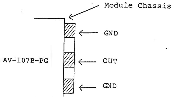
The load should be connected between the OUT and GND terminals using very short leads ( $\ll 0.5$  cm). The voltage across the load may be monitored by connecting a length of 80 mil semi-rigid 50 ohm cable as shown below (or by means of a high impedance scope probe). The current may be monitored using a current probe such as the TEKTRONIX Model CT-2.
