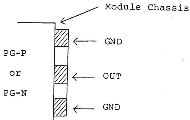
The load should be connected between the OUT and GND terminals using very short leads ( $\ll 0.5$  cm).
