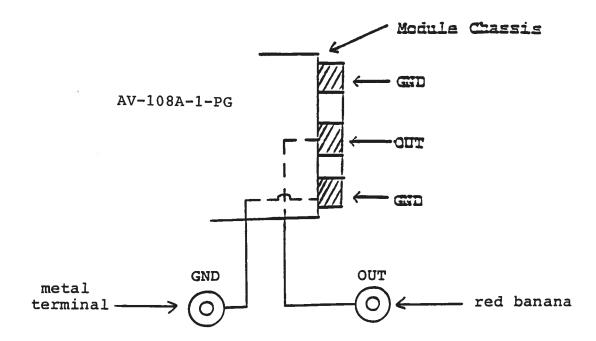
The load should be connected between the OUT and GND terminals using very short leads (≤ 10.0 cm). If the load cannot be placed directly on the output terminals of the -PG module, the AV-LZ lines should be used between the -PG module and the load (see AV-LZ data sheet). Take care to insure that during soldering the OUT conductor is not shorted to the chassis. Also, use minimal heat when soldering.
