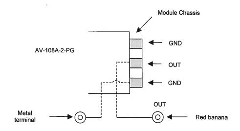
The load should be connected between the OUT and GND terminals using very short leads (≤ 10.0 cm). If the load cannot be placed directly on the output terminals of the -PG module, the AV-LZ lines should be used between the -PG module and the load (see AV-LZ data sheet). Take care to insure that during soldering the OUT conductor is not shorted to the chassis. Also, use minimal heat when soldering.
