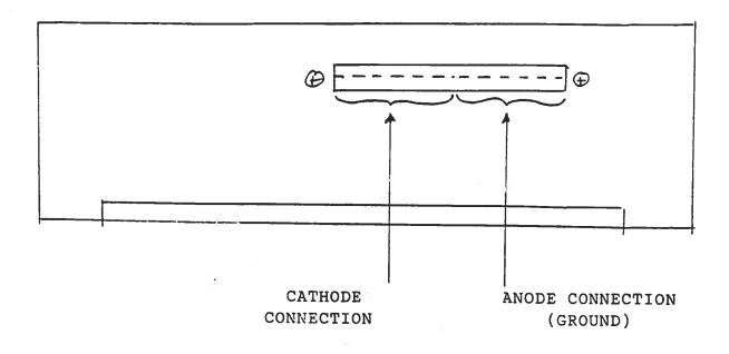
An Amp WAVECRIMP 765206-3 connector is affixed to the chassis and mates to a WAVECRIMP 765191-1 plug. The diode anode and cathode should be connected as shown in Fig. 2. The driver was tested with a 2 foot section of WAVECRIMP cable between the diode and the driver. A rise time of 8 us was observed. With a cable length of one foot, the rise time should be less than 5 us.
