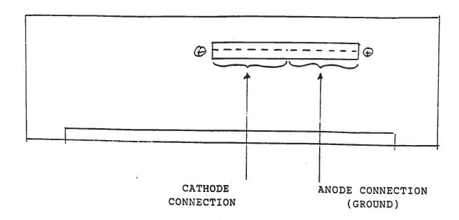
An Amp WAVECRIMP 765206-3 connector is affixed to the chassis and mates to a WAVECRIMP 765191-1 plug. The diode anode and cathode should be connected as shown in Fig. 2. The driver was tested with a 2 foot section of WAVECRIMP cable between the diode and the driver. A rise time of 8 us was observed. With a cable length of one foot, the rise time should be less than 5 us.
