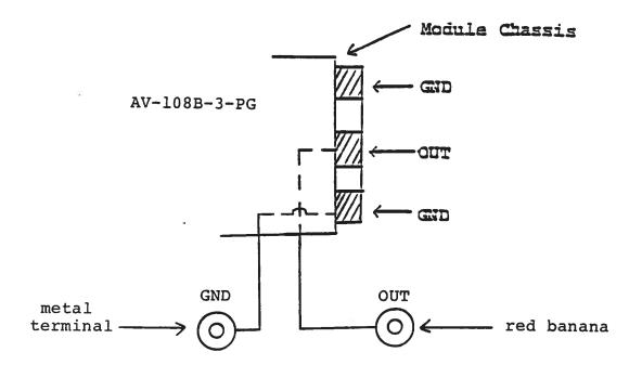
The load should be connected between the OUT and GND terminals using very short leads ( $\leq 10.0$  cm). If the load cannot be placed directly on the output terminals of the -PG module, the AV-LZ lines should be used between the -PG module and the load (see AV-LZ data sheet). Take care to insure that during soldering the OUT conductor is not shorted to the chassis. Also, use minimal heat when soldering.
