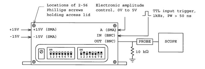
With the DIP switches set as shown, the module will trigger from the internal 30 Hz source, and will have an output pulse width of 100  $\mu s$ . The amplitude will be controlled by the Amplitude Control Pot, and the output will be noninverted.
