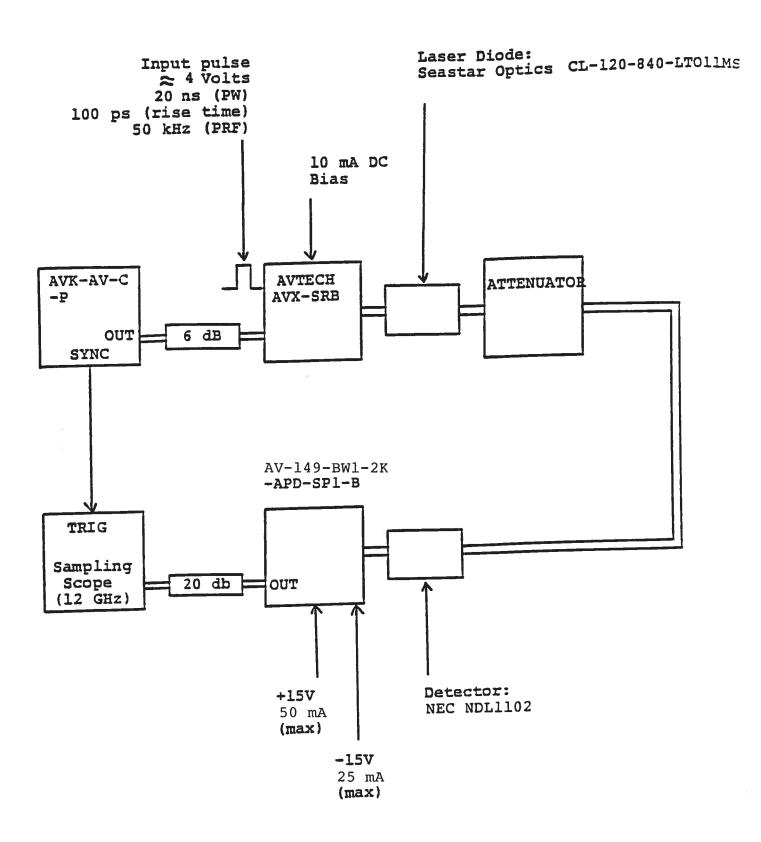
Fig. 1 BASIC TEST SET-UP (PULSE MODE)
