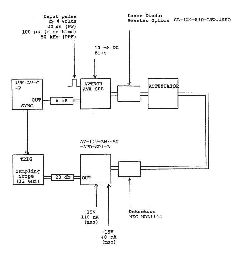
Fig. 1 BASIC TEST SET-UP (PULSE MODE)
