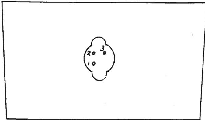
Fig. 2 DIODE SOCKET PIN CONNECTIONS
