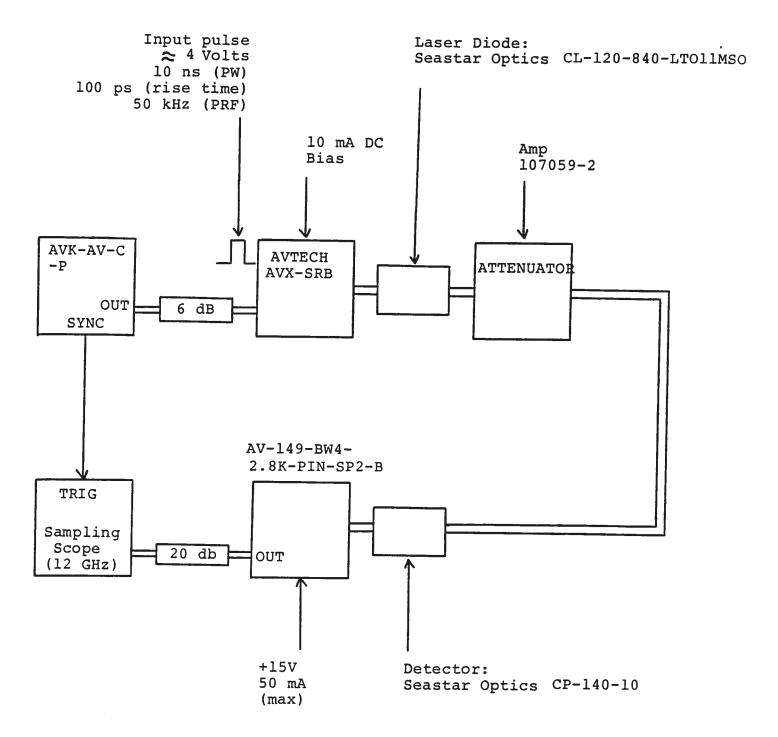
Fig. 1 BASIC TEST SET-UP (PULSE MODE)
