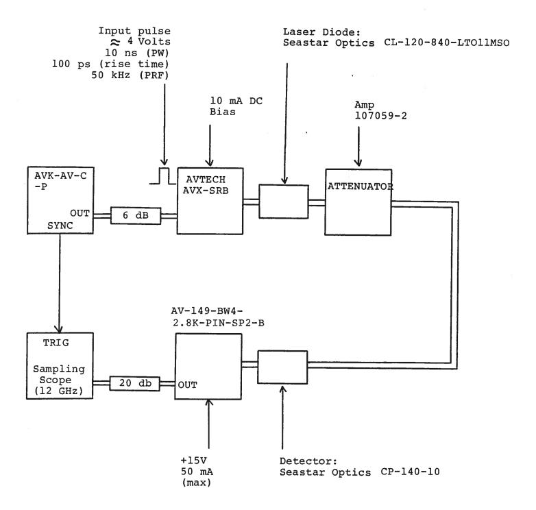
Fig. 1 BASIC TEST SET-UP (PULSE MODE)
