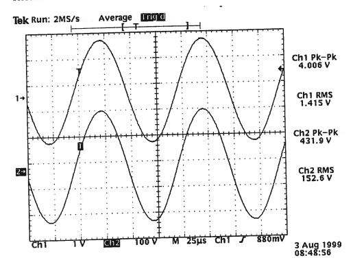
Top: 4.006 V peak-to-peak in  $(1.415 \text{ V}_{RMS})$ , 10 kHz
