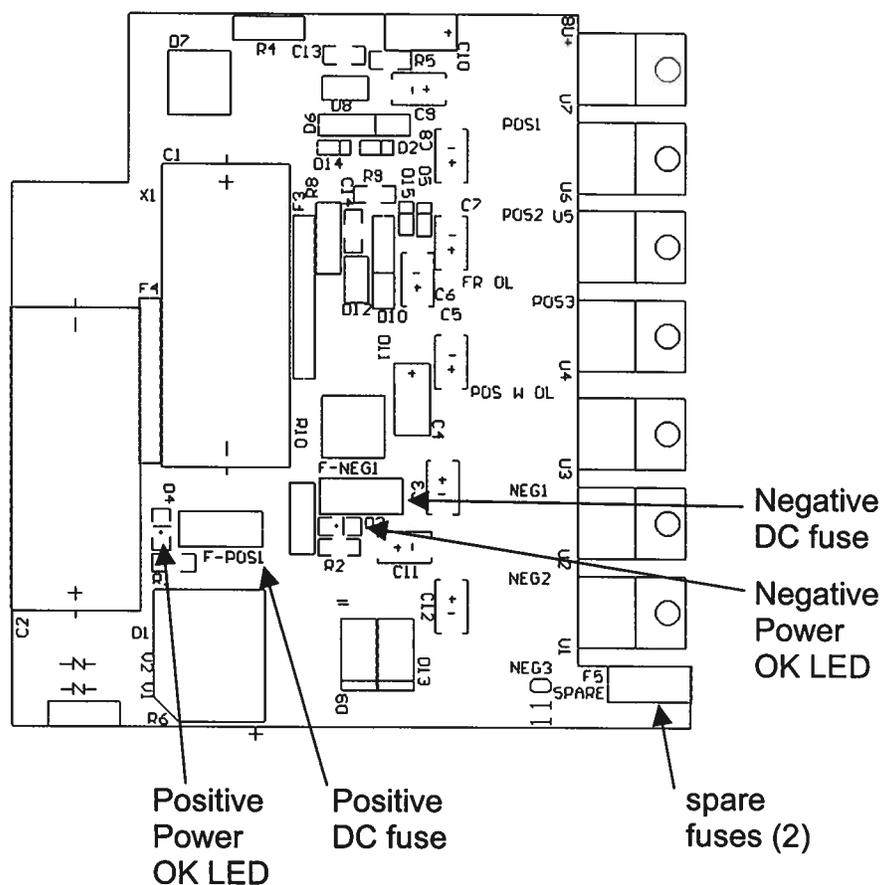
The spare fuses may be used to replace blown fuses, if required.
