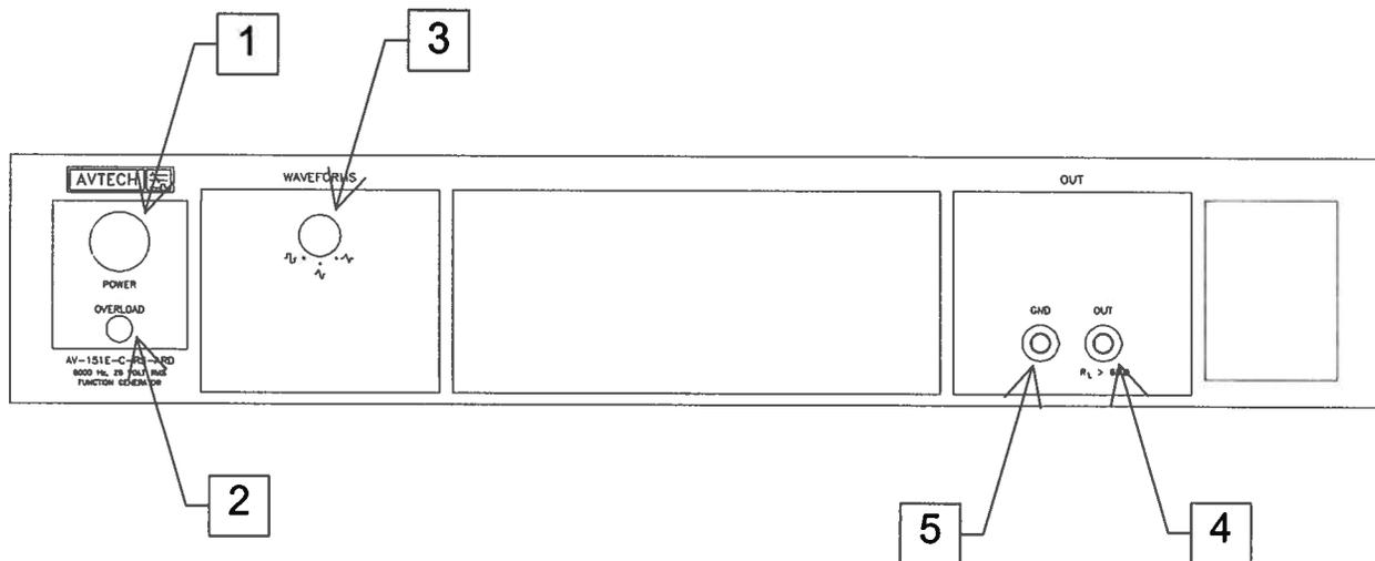
1. **POWER Switch.** The POWER push button switch applies AC prime power to the primaries of the transformer, turning the instrument on. The push button lamp (#382 type) is connected to the +15V DC supply.
