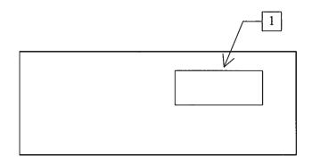
1. <u>AC POWER INPUT</u>. A three-pronged recessed male connector is provided on the back panel for AC power connection to the instrument. Also contained in this assembly is a 1A slow blow fuse and a removable card that can be removed and repositioned to switch between 120V AC in and 240V AC in.
