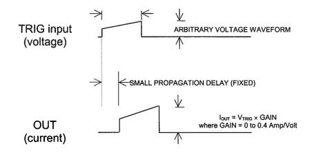
Caution: In this mode, the RMS (root mean square) output current must not exceed 1.7 Amps, and the peak output current must not exceed  $\pm 2A$ . If these limits are exceeded, the internal fuses may fail. See the "Maintenance" section for details on fuse replacement.
