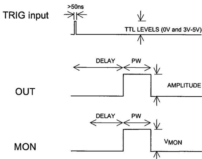
In this mode, the delay, pulse width, and amplitude of the OUT pulse can be varied with front panel controls.
