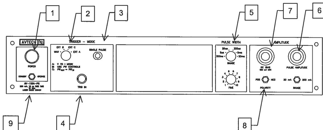
1. **POWER Switch.** The POWER push button switch applies AC prime power to the primaries of the transformer, turning the instrument on. The push button lamp (#382 type) is connected to the internal +15V DC supply.
