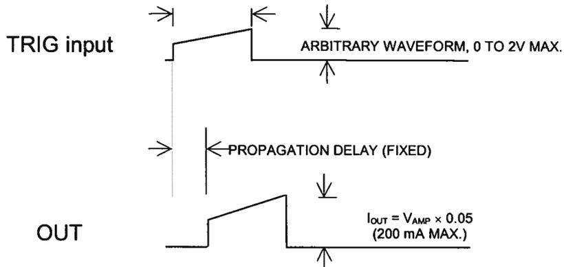
In this mode, the output pulse width and amplitude are determined by the signal on the AMP connector.
