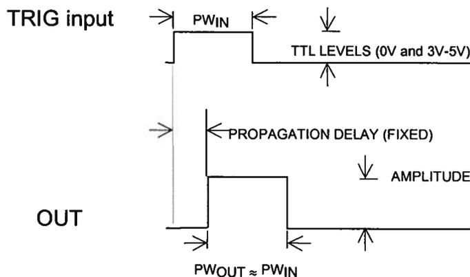
In this mode, the output pulse width is approximately equal to the pulse width of the TTL-level trigger pulse on the TRIG input. The output pulse is generated after a short propagation delay. The delay is not variable. The amplitude of the OUT pulse can be varied with front panel controls.
