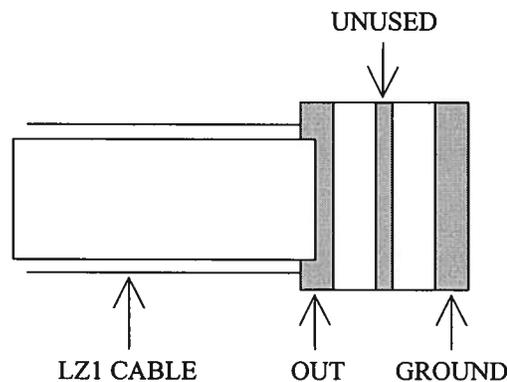
To obtain the very best waveform, it is important that the characteristic impedance of the transmission line used to connect the load to the pulser be well matched to the load impedance. This will minimize transmission line reflections.
