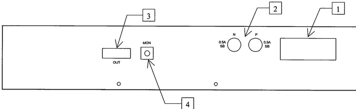
1. **AC POWER INPUT.** A three-pronged recessed male connector is provided on the back panel for AC power connection to the instrument. Also contained in this assembly is a 0.5A slow blow fuse and a removable card that can be removed and repositioned to switch between 120V AC in and 240V AC in.
