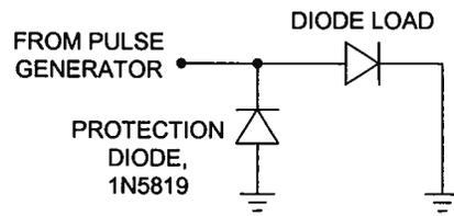
The previous diagram assumes that the diode is to be driven with a positive current. This circuit will prevent the output voltage going below approximately -0.5V.
