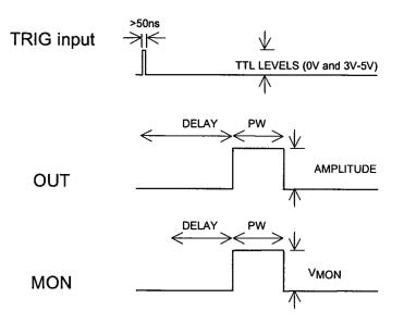
In this mode, the delay, pulse width, and amplitude of the OUT pulse can be varied with front panel controls.
