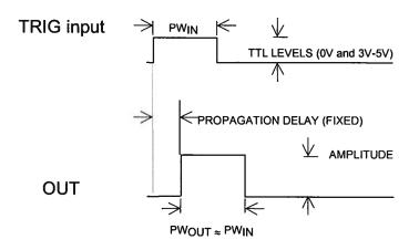
In this mode, the output pulse width is approximately equal to the pulse width of the TTL-level trigger pulse on the TRIG input. The output pulse is generated after a short propagation delay. The delay is not variable. The amplitude of the OUT pulse can be varied with front panel controls.
