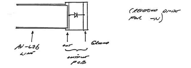
For units with the S5 option, the diode plugs directly into the socket provided.
