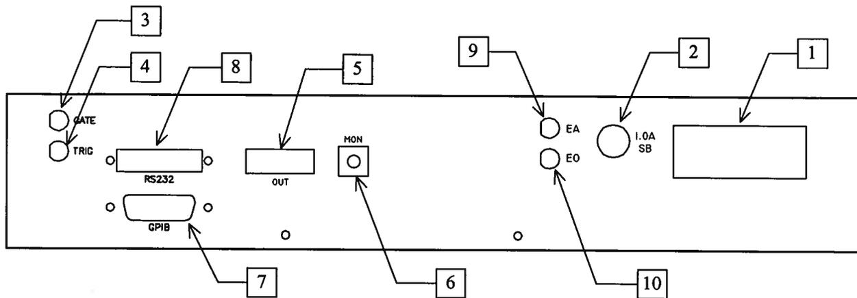
1. **AC POWER INPUT.** A three-pronged recessed male connector is provided on the back panel for AC power connection to the instrument. Also contained in this assembly is a 2.0A slow blow fuse and a removable card that can be removed and repositioned to switch between 120V AC in and 240V AC in.
