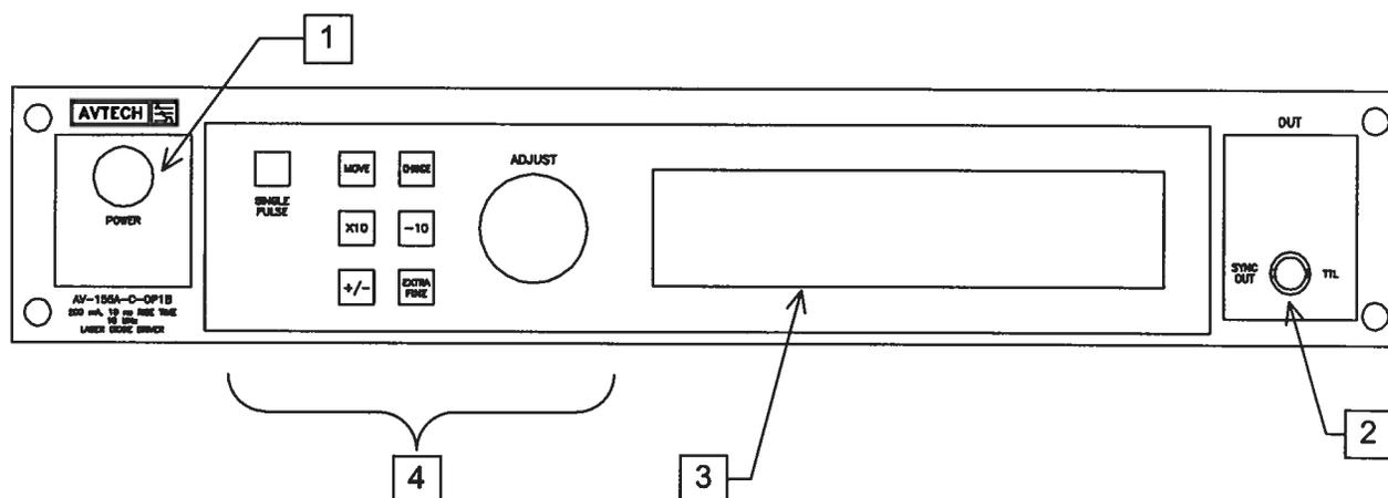
1. **POWER Switch.** The POWER push button switch applies AC prime power to the primaries of the transformer, turning the instrument on. The push button lamp (#382 type) is connected to the +15V DC supply.
