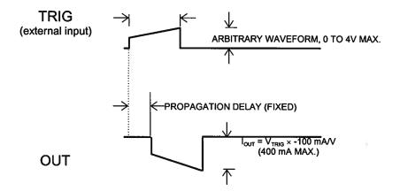
In this mode, the output pulse width and amplitude are determined by the signal on the TRIG connector. Note that a SYNC pulse is only generated if the TRIG input exceeds approximately 2V (i.e. a TTL-level logic high).
