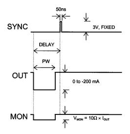
Basic Output Pulses for Delay < 0
