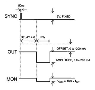
Basic Output Pulses for Delay > 0
