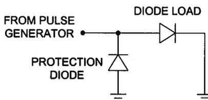
This will prevent the output voltage from falling below approximately -0.7V.
