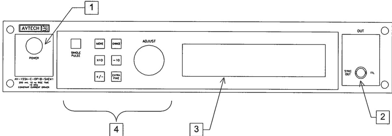
1. **POWER Switch.** The POWER push button switch applies AC prime power to the primaries of the transformer, turning the instrument on. The push button lamp (#382 type) is connected to the +15V DC supply.
