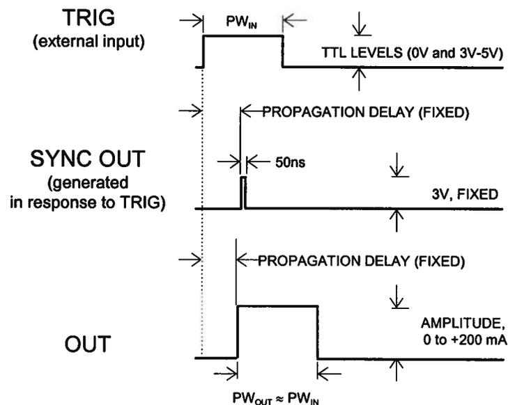
In this mode, the output pulse width is approximately equal to the pulse width of the TTL-level trigger pulse on the TRIG input. The output pulse is generated after a short propagation delay. The delay is not variable. The amplitude of the OUT pulse can be varied with front panel controls or via the GPIB or RS-232 computer interfaces.
