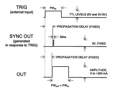
In this mode, the output pulse width is approximately equal to the pulse width of the TTL-level trigger pulse on the TRIG input. The output pulse is generated after a short propagation delay. The delay is not variable. The amplitude of the OUT pulse can be varied with front panel controls or via the GPIB or RS-232 computer interfaces.
