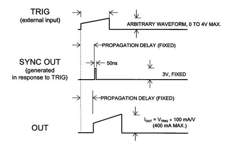
In this mode, the output pulse width and amplitude are determined by the signal on the TRIG connector. Note that a SYNC pulse is only generated if the TRIG input exceeds approximately 2V (i.e. a TTL-level logic high).
