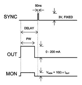
Basic Output Pulses for Delay < 0
