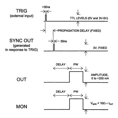
In this mode, the delay, pulse width, and amplitude of the OUT pulse can be varied with front panel controls or via the GPIB or RS-232 computer interfaces.
