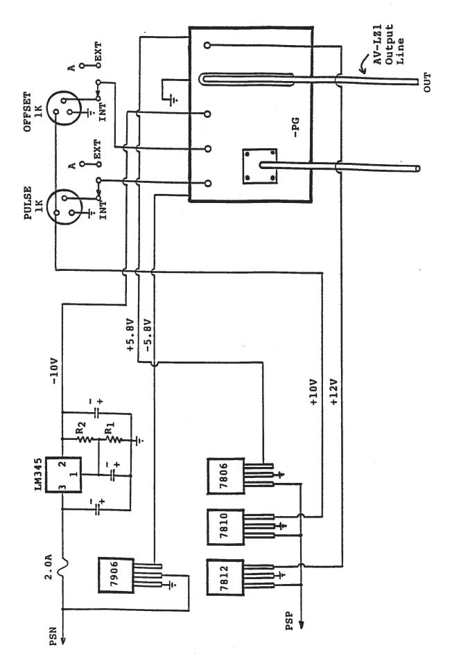
Fig. 5: AV-155-PS-DUP3 BLOCK DIAGRAM
