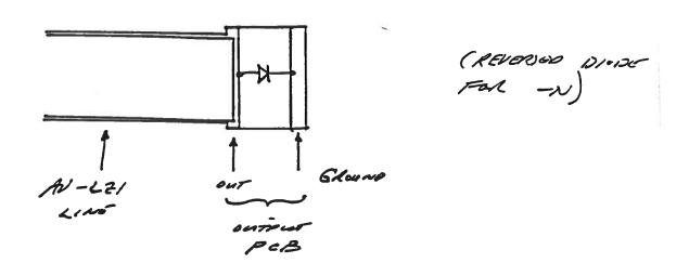
For units with the PUl option, a BNC connector is connected to the output PCB. If a cable is connected to this connector (with the laser diode between the center conductor and ground), the cable may serve to distort the pulse and the degree of distortion will increase with the cable length.
