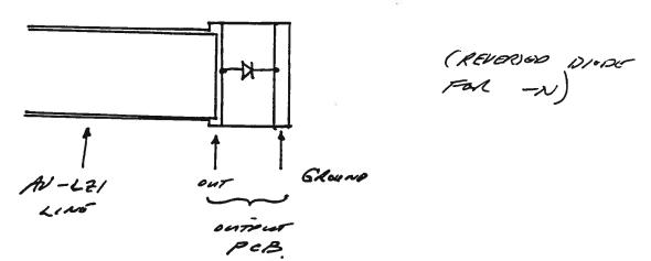
For units with the S5 option, the diode plugs directly into the socket provided.
