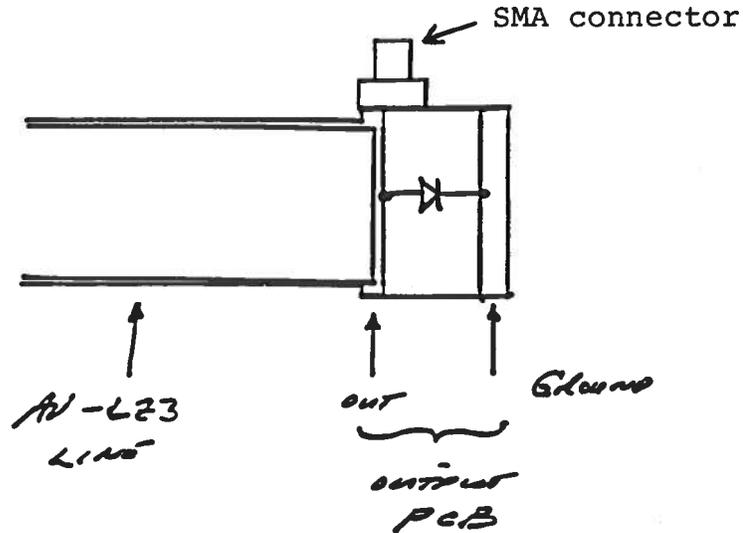
As with the resistive load, the laser diode may also be placed at the end of a 30 cm 50 Ohm cable which connects to the SMA connector on the small PCB output board.
