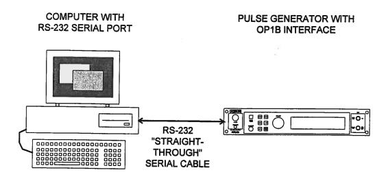
The computer is connected with a RS-232 "straight-through" cable. This cable is available at most computer stores, and it is the same type of cable that is generally used to connect a PC to an external modem. Beware that newer PCs generally have 9-pin male RS-232 connectors, whereas older computers generally have 25-pin male RS-232 connectors. The actual cable wiring connections are described in the "Cable Connections" section.
