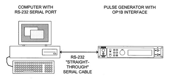
The computer is connected with a RS-232 "straight-through" cable. This cable is available at most computer stores, and it is the same type of cable that is generally used to connect a PC to an external moder. Beware that newer PCs generally have 9-pin male RS-232 connectors, whereas older computers generally have 25-pin male RS-232 connectors. The actual cable wiring connections are described in the "Cable Connections" section.
