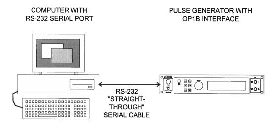
The computer is connected with a RS-232 "straight-through" cable. This cable is available at most computer stores, and it is the same type of cable that is generally used to connect a PC to an external modern. Beware that newer PCs generally have 9-pin male RS-232 connectors, whereas older computers generally have 25-pin male RS-232 connectors. The actual cable wiring connections are described in the "Cable Connections" section.
