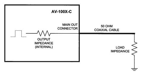
However, to obtain output amplitudes greater than  $\pm 5V$ , the  $\pm 10V$  ranges must be used, and the output impedance will be  $2\Omega$ . This is slightly less ideal, but good waveforms will still be obtained since the transmission line is still properly terminated on one end (the load end) with  $50\Omega$ .
